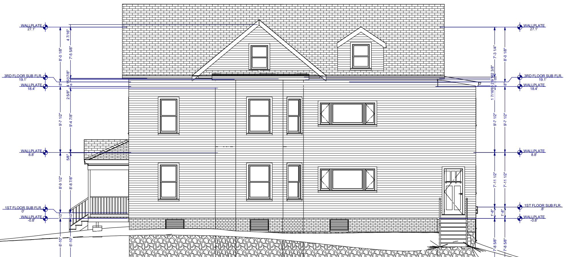
EXISTING CONDITIONS - RIGHT ELEVATION SCALE: 1/8" = 1'-0"
